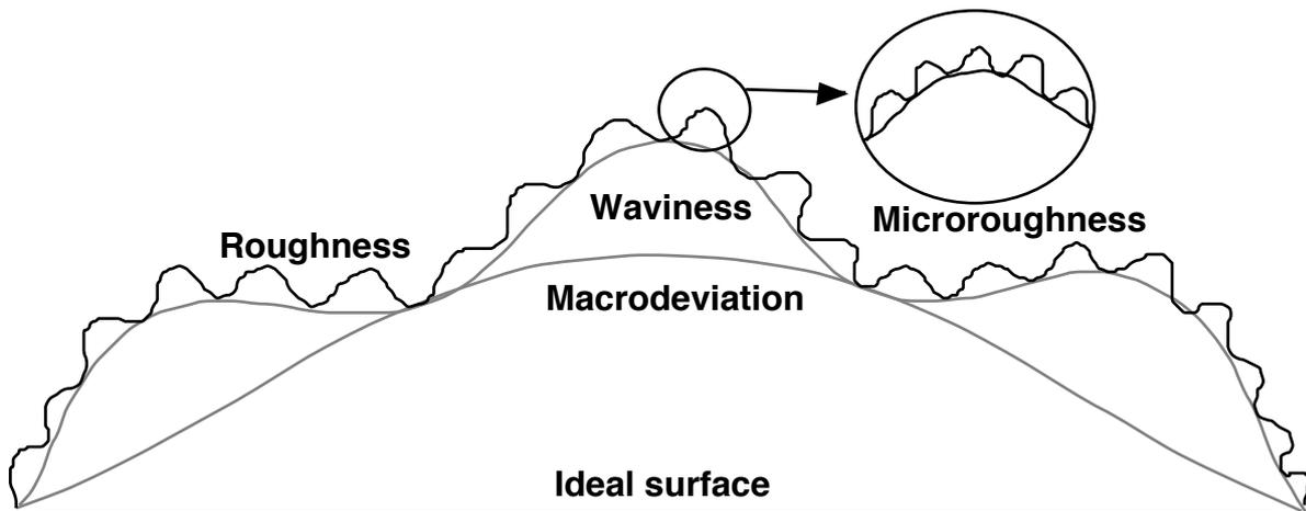
Fig. 1 Schematic sketch of macrodeviation, Waviness, roughness and microroughness.
