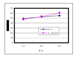
The curves cross at d/w = 0.2, i.e. d = 8 mm. However, the crossing is shallow meaning that a small change in conditions results in large changes in the hole diameter.
