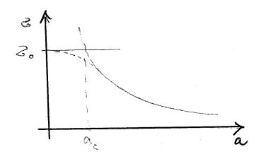
Brittle fracture occurs when  $K_{IC} = \sigma 1.12 \sqrt{\pi a}$  For small cracks ductile tearing occurs when  $\sigma = \sigma_0$ . An approximate crack length marking the change from brittle to ductile fracture is obtained from  $K_{IC} = \sigma_o 1.12 \sqrt{\pi a_c}$
