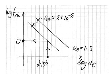
The joint class C is the stress range for which the welded joint can sustain the fatigue life  $n_{\rm t} = 2 \cdot 10^6$  cycles with the risk of failure  $Q_{\rm B} = 0.023$  (2 standard deviations shift of the median curve for the welded joint).
