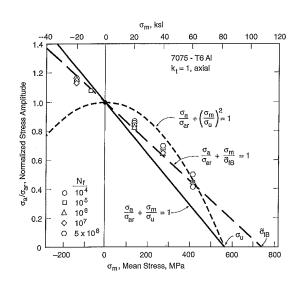
See Dowling p 429. The equivalent completely reversed stress amplitude  $\sigma_{ar}$  is defined on Dowling p 431. We have for the Modified Goodman equation (9.17) and Smith-Watson-Topper (SWT), (9.18) respectively
