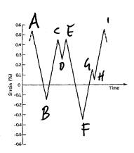
Use Dowling p 446-447. Inserting strain values we identify cycles as:
