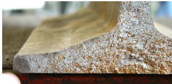
(b) Geometry of a rail foot crack that caused a rail break.
