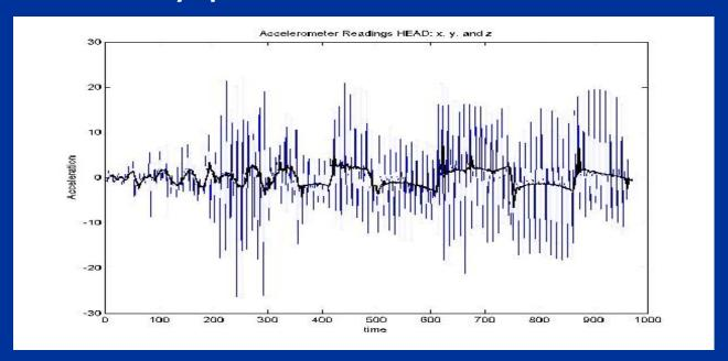
Noise: Real sensors (and actuators) are noisy
