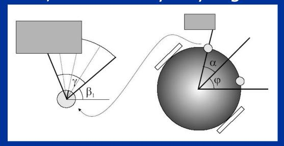
$\varphi$  is current heading of the robot,  $\alpha$  is relative direction of the IR sensor, and  $\gamma$  is opening angle of sensor
